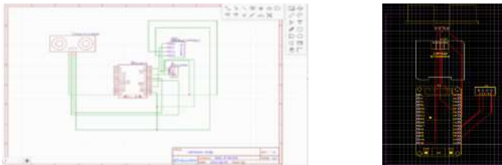
Figure 8. Circuit connection of Ultrasonic range meter
